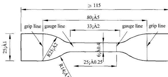
Fig 1. Dumbbell shaped specimen
