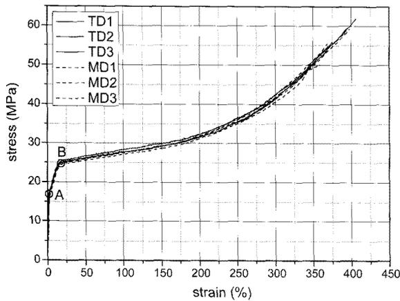
Fig 3. Stress strain curves of ETFE film
